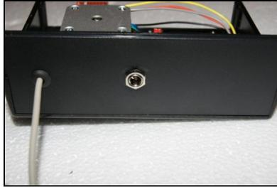
Insert the front panel into the grooves into the top panel.
