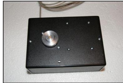
Install 4 rubber feet on the bottom of the case at each CORNER.
