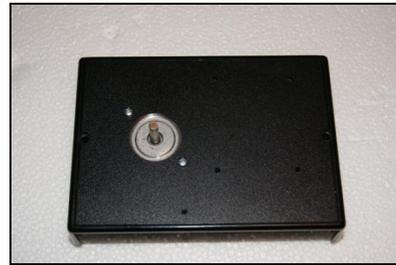
Install the hub flush over the top of the step motor shaft. Do not force but slide the hub over the shaft in a docile manner. Tighten the set screw. Make sure that the hub and case do not touch. Apart from the slight stepper motor resistance when turned by hand the motor shaft/hub should turn easy.
